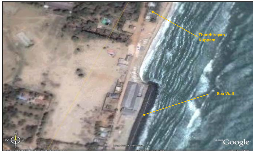
Figure 4: As sea wall ends, erosion begins
