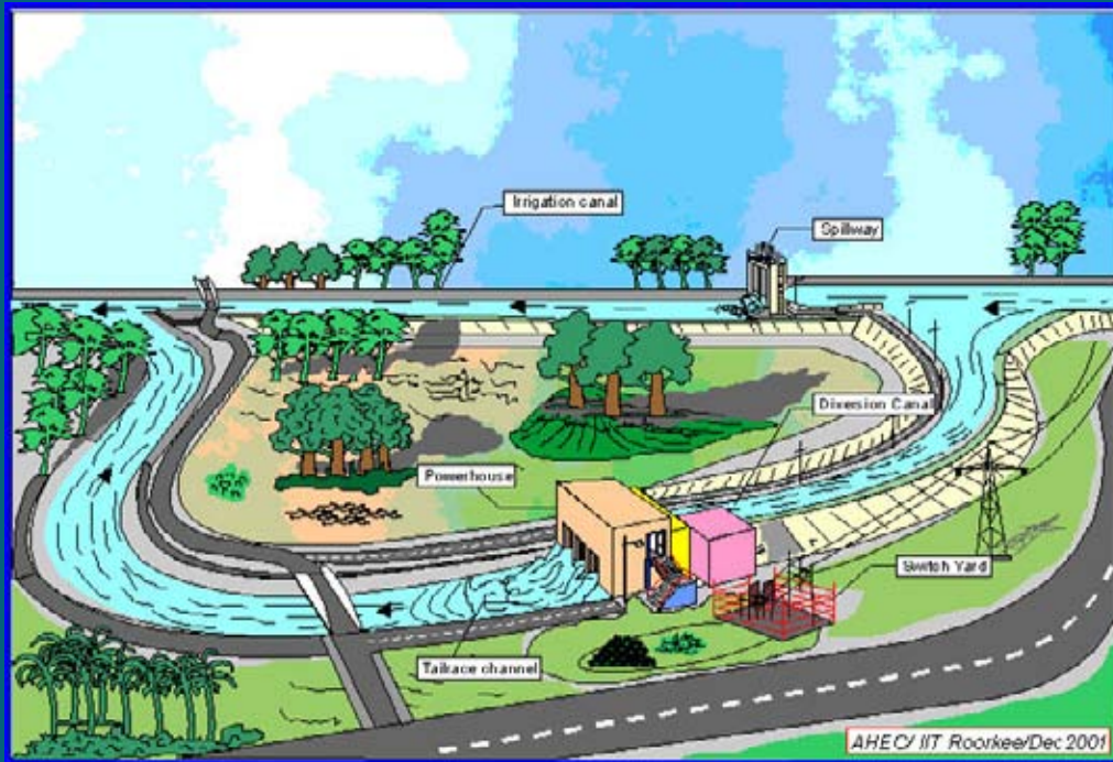
Typical Arrangement of Canal Fall Small Hydro Power Station
