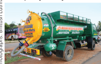
Vacuum tanker with 5,000 litre capacity (Trichy)
