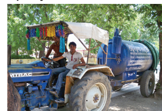
Vacuum tanker with 5,000 litre capacity (Trichy)
