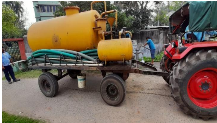
Figure 6: Transportation of FS by Vacuum Tanker, source: Akansha/CSE, 2020
