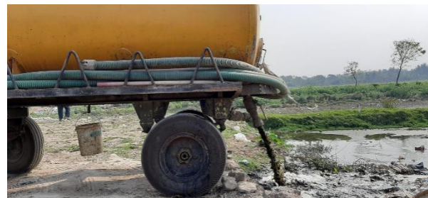
Figure 7: Discharge of Faecal Sludge into open ground (Source: Manish/CSE, 2020)
