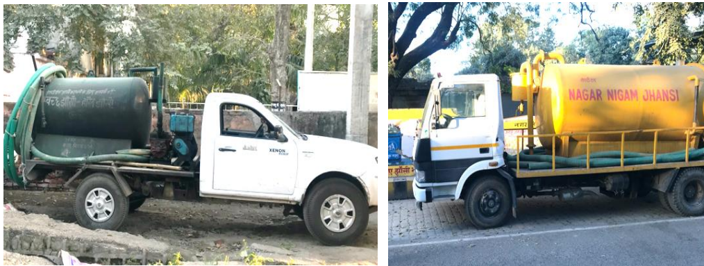
Figure 9: Vacuum Trucks 1500 L and 600 L owned by JNN (Source: Shrutaswinee/CSE, 2020)
