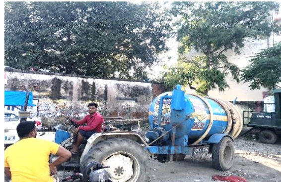
Figure 7: Tractor Mounted Vacuum Emptying Tanker (Harsh/CSE,2020)
