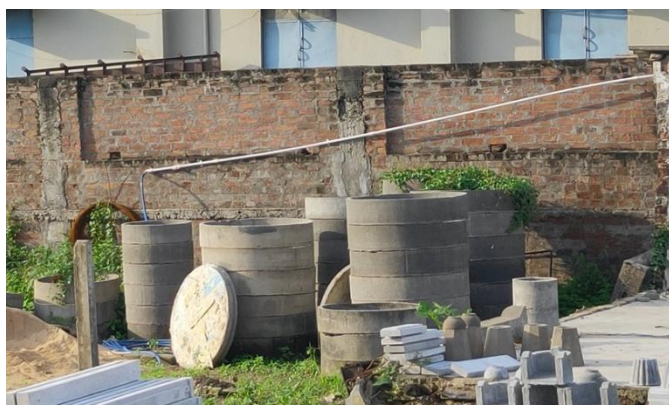
Figure 1: Cement Rings used for lined pits
