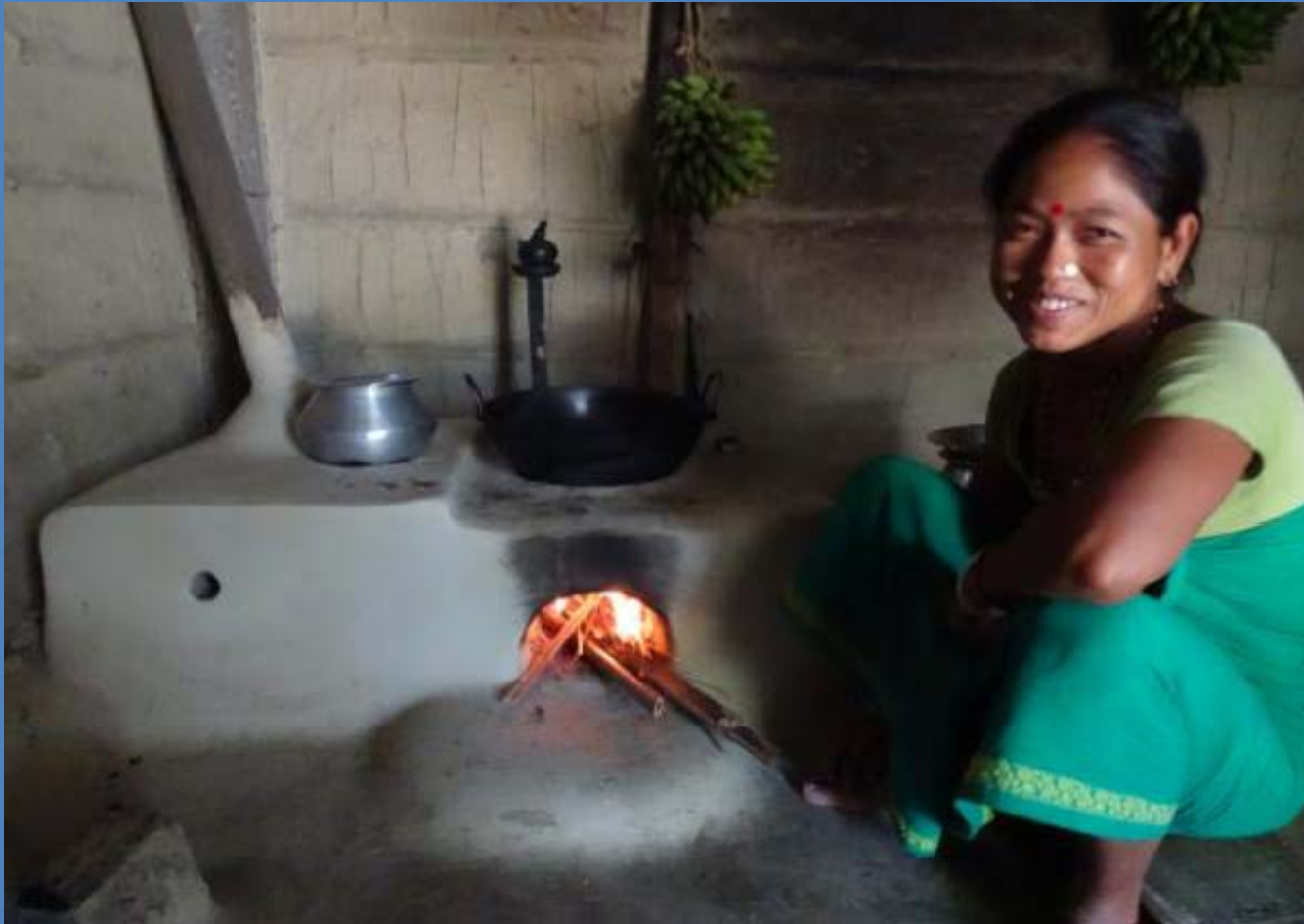
Fig: A view of improved cookstove installed two years back in 2012; fuelwood consumption reduced by~ 30%
