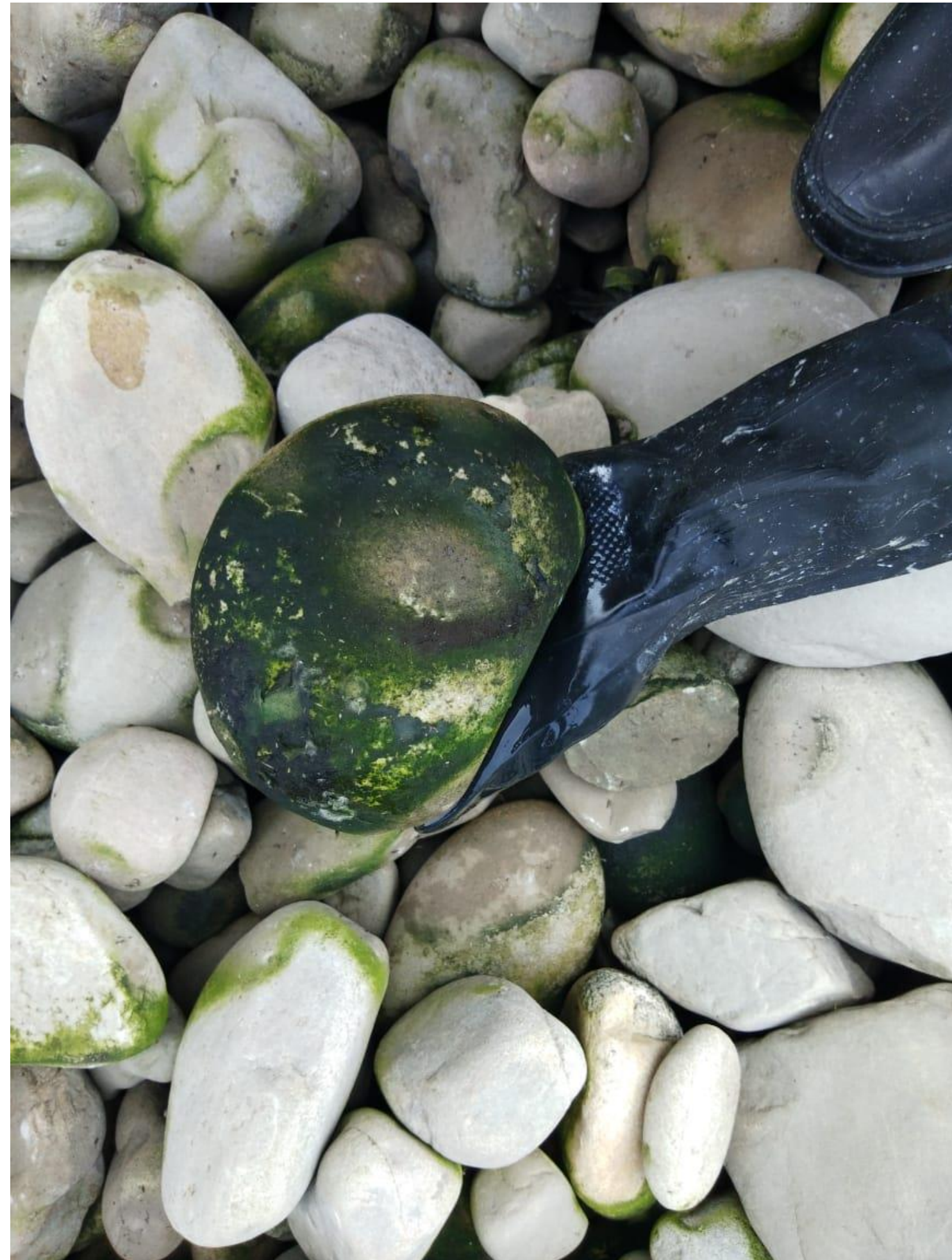
BEFORE CLEANING: Algae growth on stones in PGF
