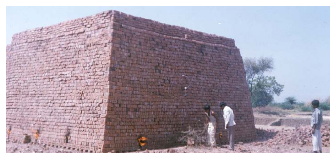
Firing Technology - Clamps Share – 25 % of India production Fuel – Biomass (80%) & Coal (20%)
