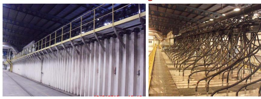
Tunnel Kiln – 145 m. long – 5.0 m width – Most efficient technology at work
