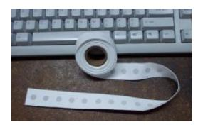
Aethalometer relates changes in transmission through filter paper to the load of black carbon particles.
