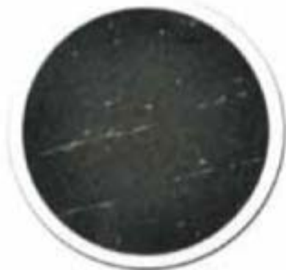
No retrofit system Uncontrolled Diesel Exhaust (Level 1)
