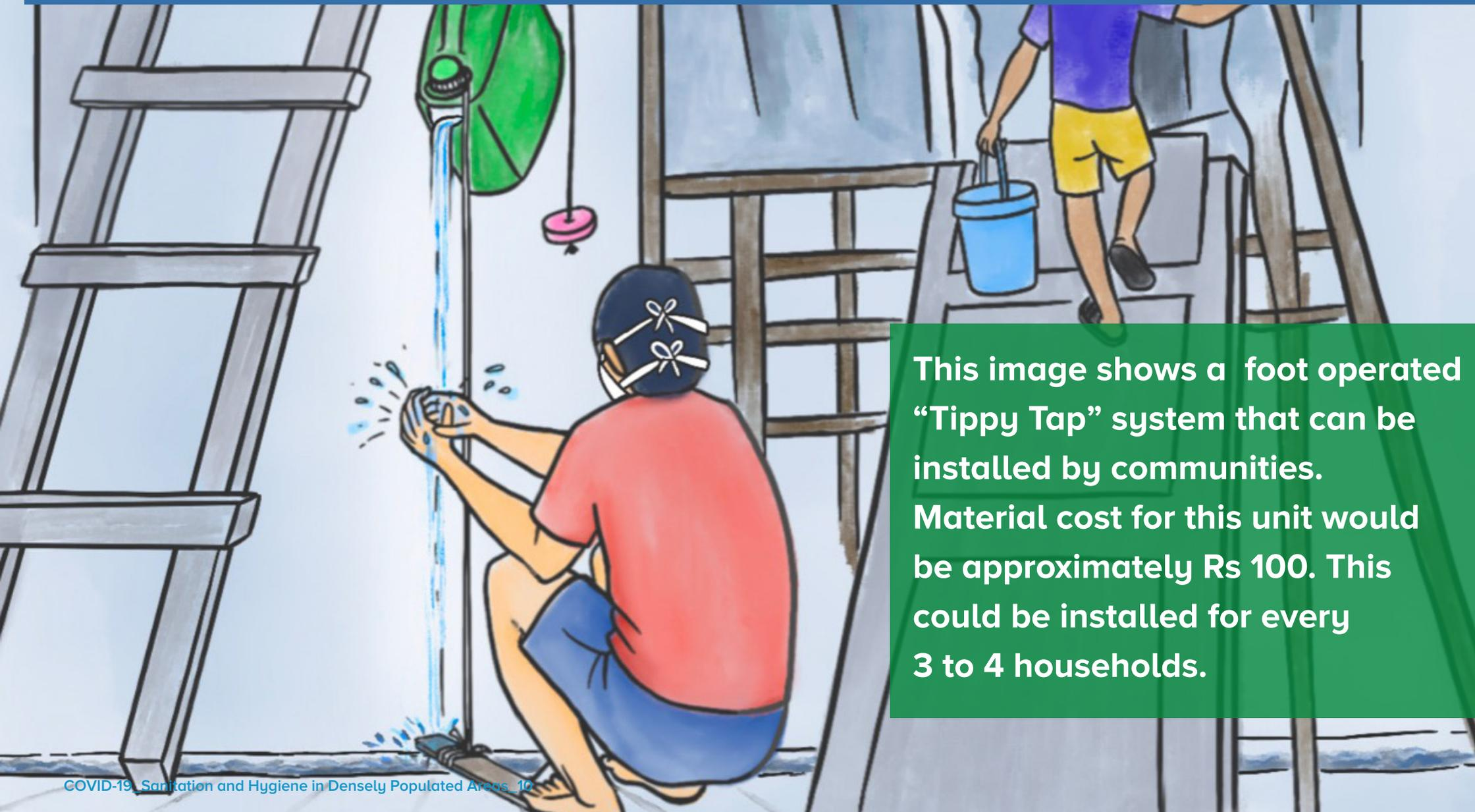
This image shows a foot operated “Tippy Tap” system that can be installed by communities. Material cost for this unit would be approximately Rs 100. This could be installed for every 3 to 4 households.
