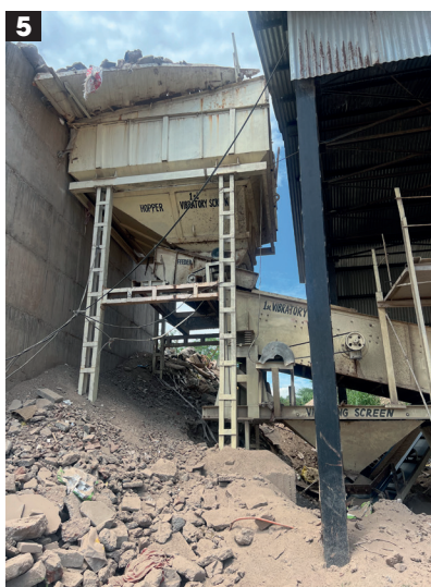
5, 6 and 7: C&D plant: Dry processing equipment (in sequence)
