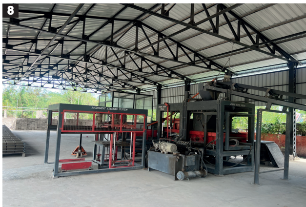
8. Automatic block making machine
