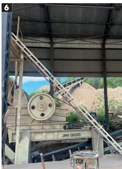
5, 6 and 7: C&D plant: Dry processing equipment (in sequence)
