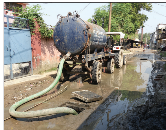
Figure 4: Tractor mounted vacuum tank owned by the NPP.
