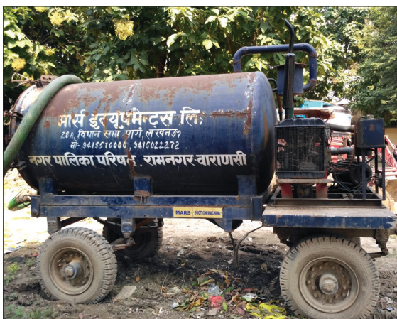
Figure 3: Vacuum tanker emptying/cleaning sewer manholes.
