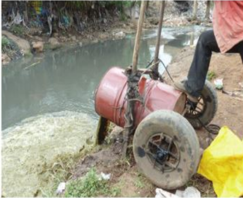
Figure 3: Manual emptier discharging the collected faecal sludge in a nearby stream ©GIZ/Doreen Mbalo
