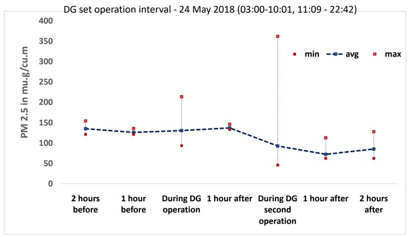
• PM2.5 max levels increased from 150 to 220 ug/N.cu.m and avg. levels almost similar.
