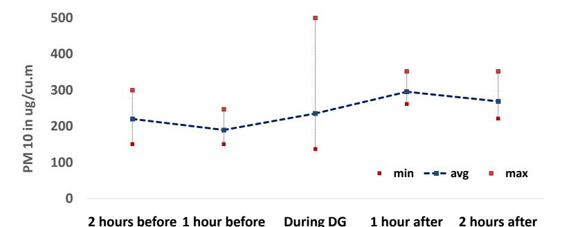
PM10 max levels increased from 250 to 500 ug/N.cu.m during DG operations, post
