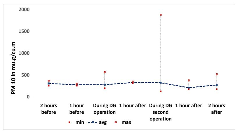
PM10 max levels increased from 250 to 500 ug/N.cu.m during DG operations, post DG operations the levels remained ~300 mg/N.cu.m over 2 hrs.
