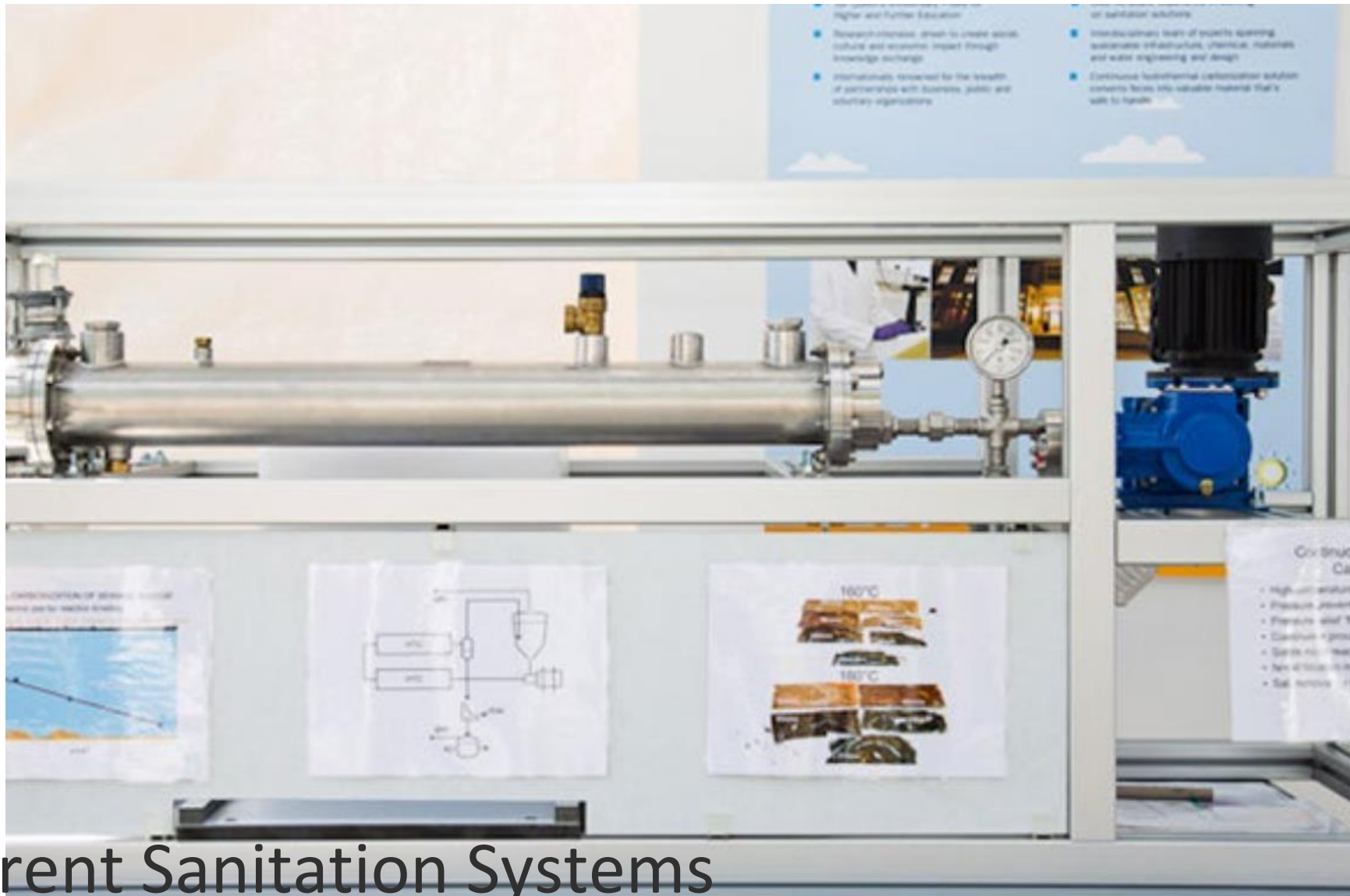
Toilet that produces biological charcoal, minerals, and clean water through hydrothermal carbonization
