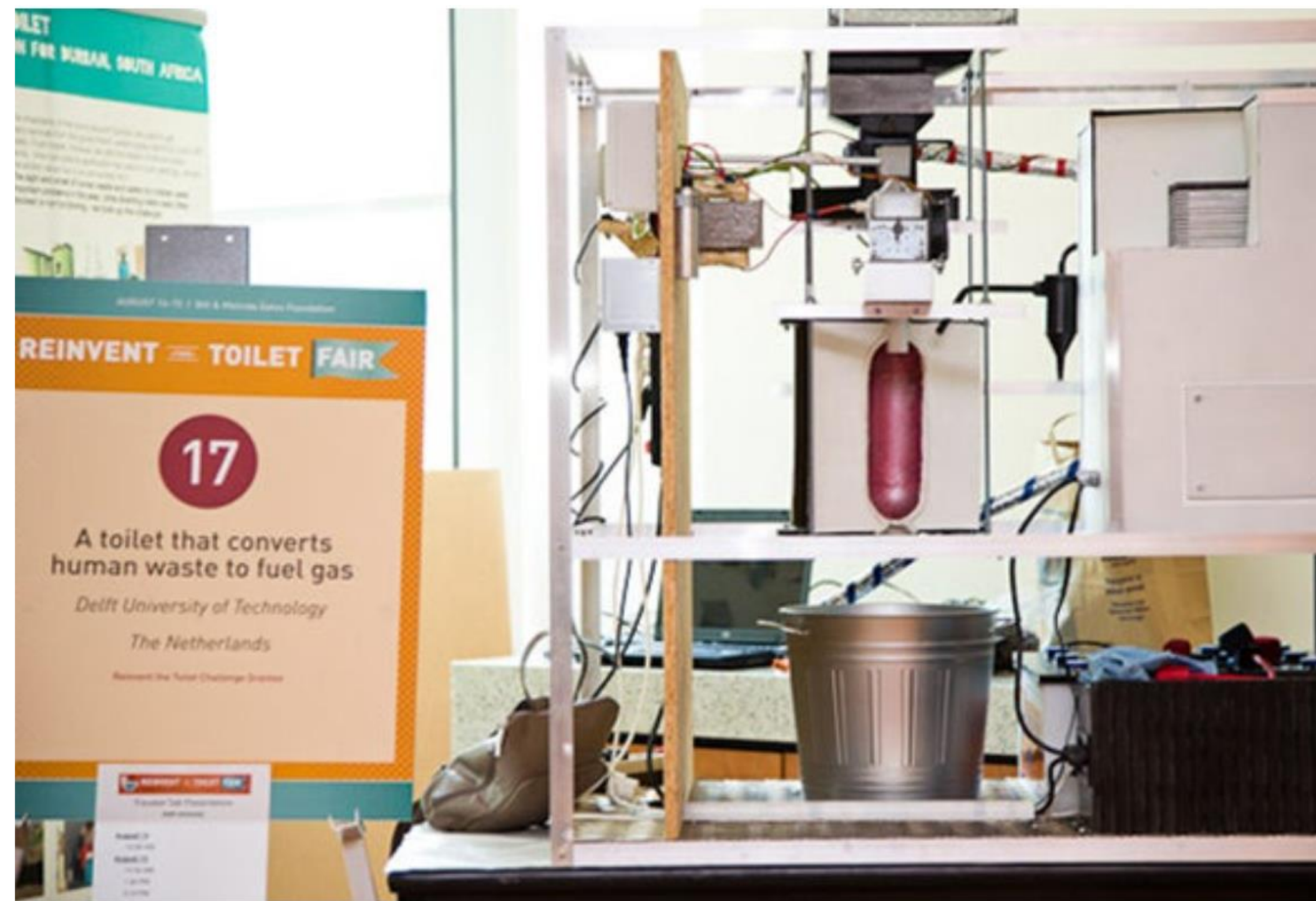
Toilet that converts human waste to fuel gas using microwaves
