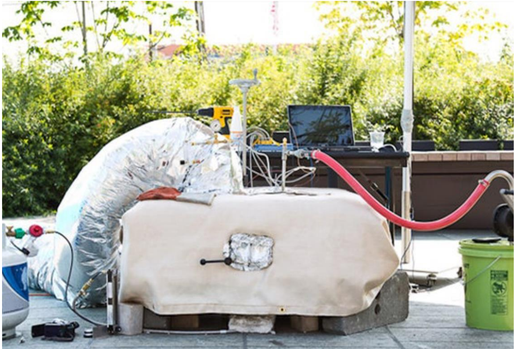
A sanitation system that converts human waste into biological charcoal
