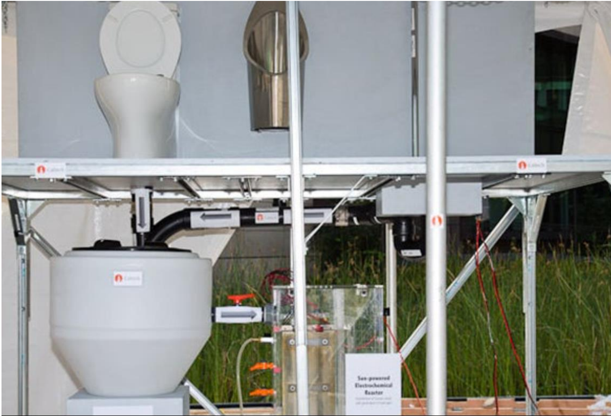
Solar-powered toilet that generates hydrogen and electricity
