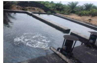
Separation tank used to collect the light pyrolysis oil at the top and the heavier residues
