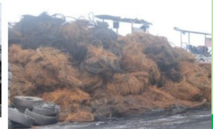
Steel recovered from pyrolysis of waste tyres
