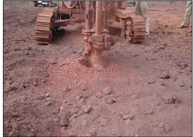
DRILLING MACHINE EQUIPPED WITH WET DRILLING PROVISION
