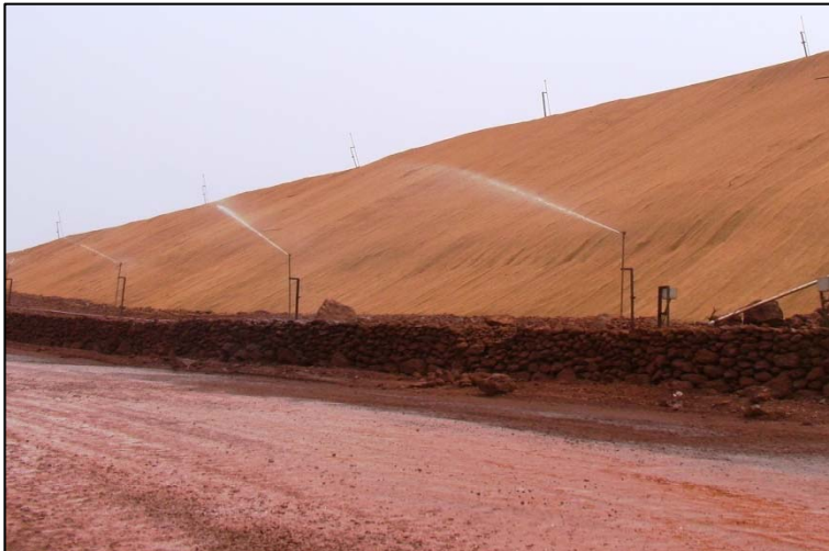
FIXED AUTO SPRINKLERS FOR MINERAL DISPATCH ROADS
