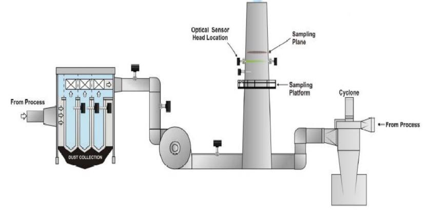
Positions to be considered for installation of Particulate Monitors
